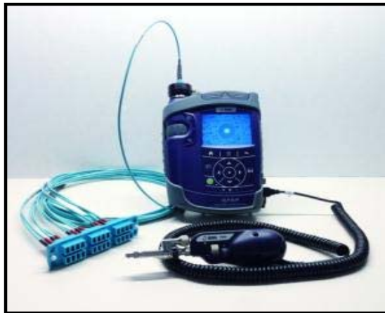
Patch Cord (“Male”) Inspection
