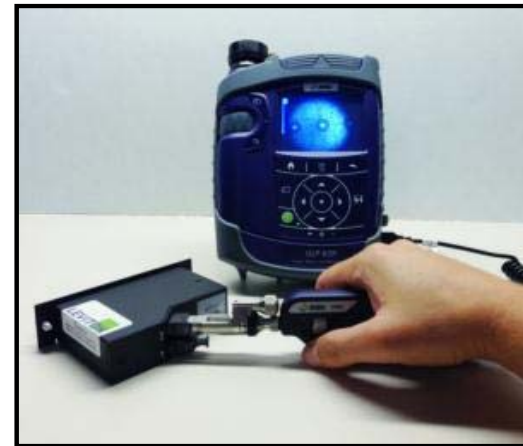
Bulkhead (“Female”) Inspection
