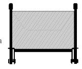
Cable Runway with optional retaining posts Usable area is runway width multiplied by maximum height of \*6"
