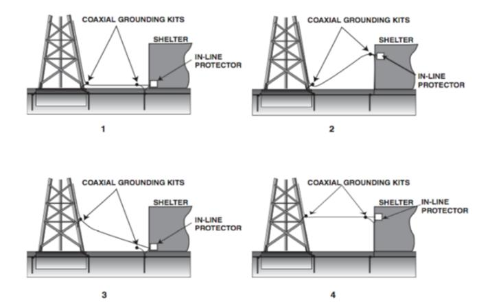
If the soil is a perfect ground, then reducing the distance from coax grounding kits to the soil-ground at the tower is the key!
