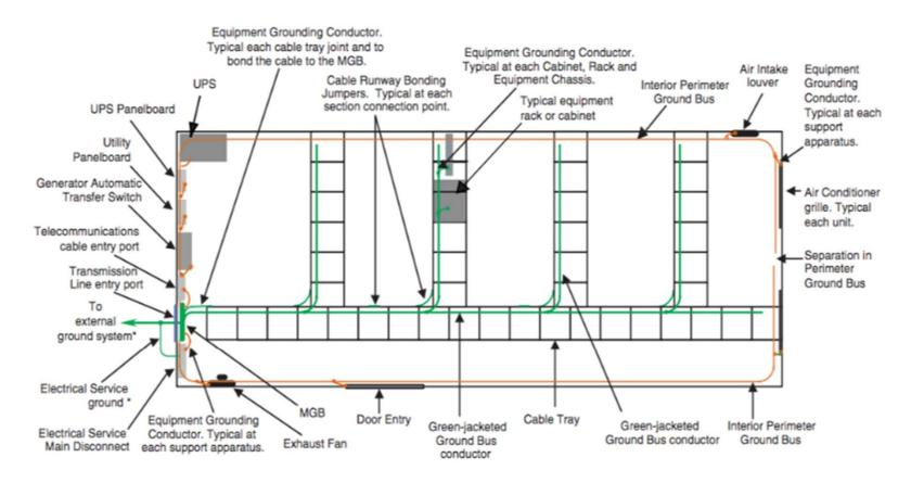
NOTE: No exterior ground system conductors shown. Electrical service grounding electrode conductor must be bonded to external site ground system.
