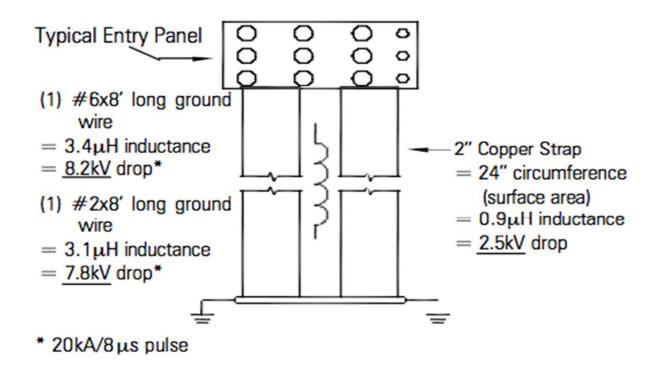
1,000V of potential/one foot of round conductor above ground.
