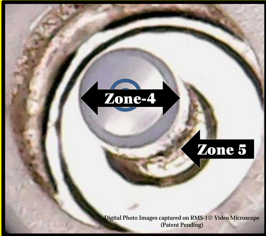
This connector “passes” all existing standards and tests: it’s contaminated on unseen surface ‘geometry’.
