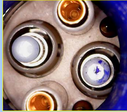
2.) Fiber was dyed. Note Zone-4 contamination extending to Zone-5
