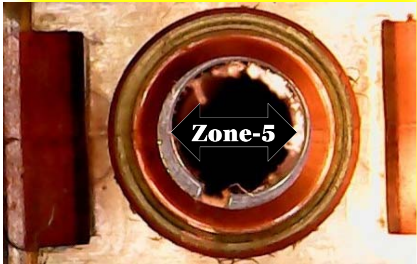
Adapter & Alignment Sleeve Contamination (unseen surface 'geometry')
